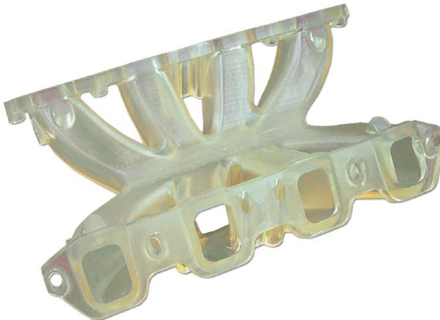
Automotive intake manifold used for fit checking and performance testing
